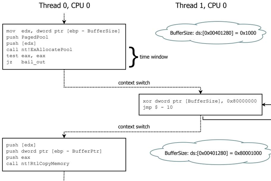
Figure 3: Context switch order allowing exploitation of a double-fetch vulnerability on a single CPU.
